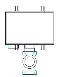
EPOXY COATING STAINLESS STEEL CONSTRUCTION ⊐SEDIMENT BASKET 🗀 FILTER MEDIA DRAW OFF VALVE ALTERNATE INLET & DUTLET SIZE \_\_\_\_ INCHES
