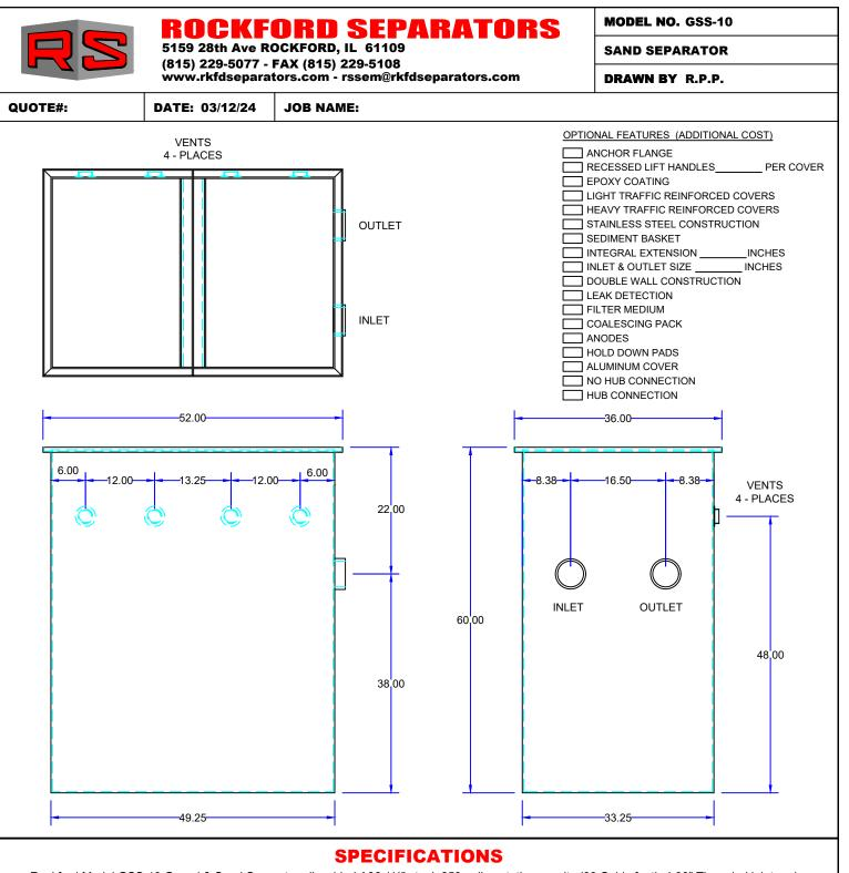
Rockford Model GSS-10 Gravel & Sand Separator all welded A36 1/4" steel, 250 gallon static capacity (33 Cubic feet), 4.00" Threaded inlet and outlet, 2.00" threaded vent connections (4), removable filter screen, non-removable baffle plates, (2) 3/8" nonskid diamond tread plate cover (for flush-with- floor installation) for pedestrian traffic, secured with stainless steel flat head screws, heavy duty leak proof gasket, OPEX SHOP COAT coating inside & bituminous coating outside.
