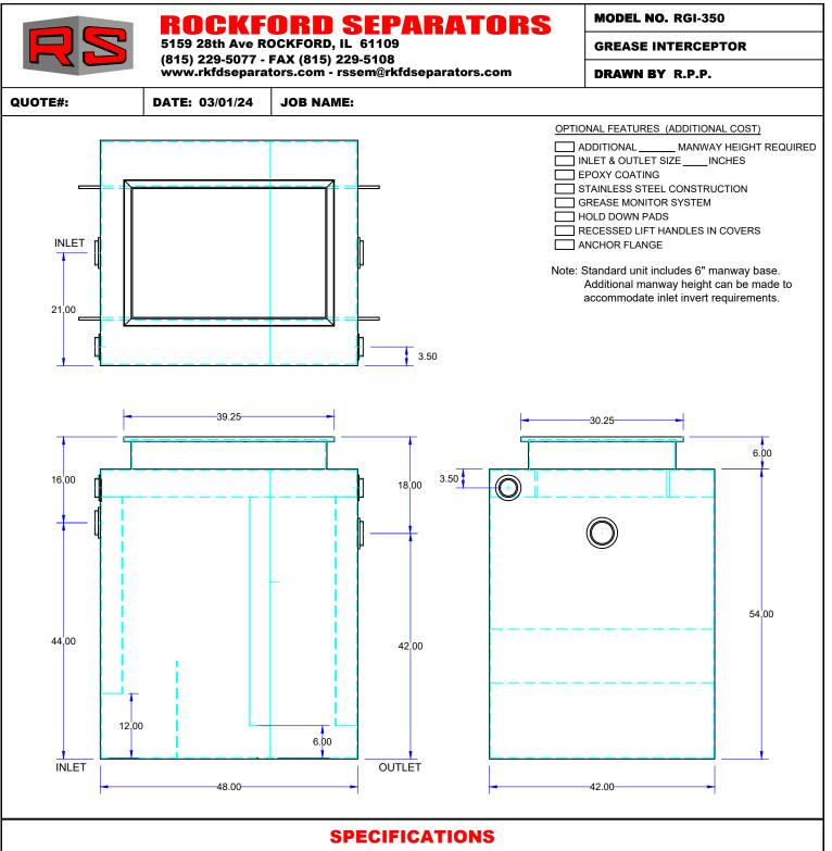
Rockford Model RGI-350 all welded steel gravity grease interceptor, with 200 intermittent GPM, 350 gallon capacity, 817 LBS greasy sludge capacity, 4" threaded inlet/outlet and 3" vent connections, removable 3/8" nonskid tread plate cover for flush with grade installation suitable for heavy traffic load (H/20), secured with stainless steel flat head screws, heavy duty leak proof gasket, with bituminous coating outside. Supplied with lifting lugs X4. Approximate ship weight of 1200 Lbs.
