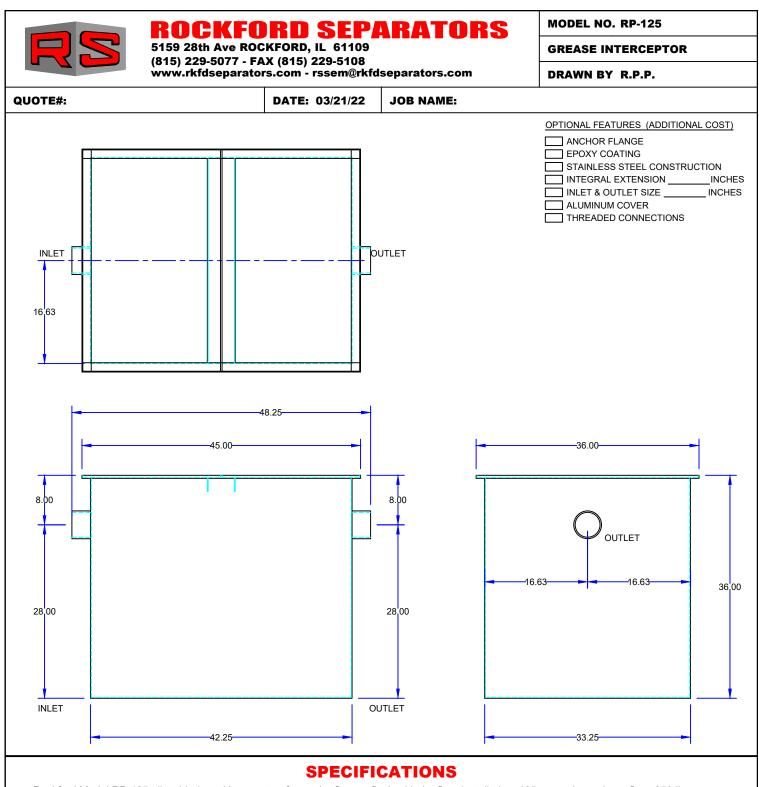
Rockford Model RP-125 all welded steel interceptor, for on the floor or flush with the floor installation, 125 g.p.m. intermittent flow, 250 lbs. grease capacity, 4.00" no-hub inlet and outlet connections and flow control device, removable 3/16" nonskid diamond tread plate cover for on the floor or flush with floor installation suitable for pedestrian traffic, secured with stainless steel flat head screws, heavy duty leak-proof gasket, enamel coating inside and outside
